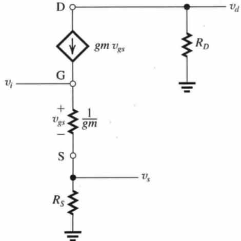
$$v_i = (g_m v_{gs}) \left( \frac{1}{g_m} + R_S \right)$$
